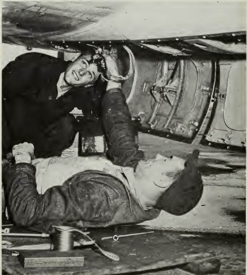
RESERVE CREWMEN work behind scenes to keep their planes on the prowl. Above: AO installs practice depth bomb. Below: Plane's wiring is checked.
